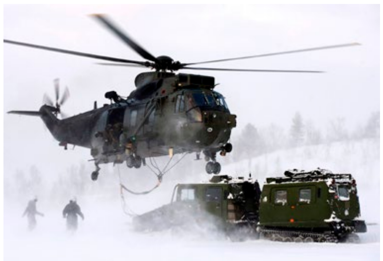
Royal Navy Sea King Mk4 helicopter pilots and aircrews carry out a load lifting exercise in Norway
